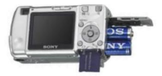
Remove the 2 AA batteries and Media Card
